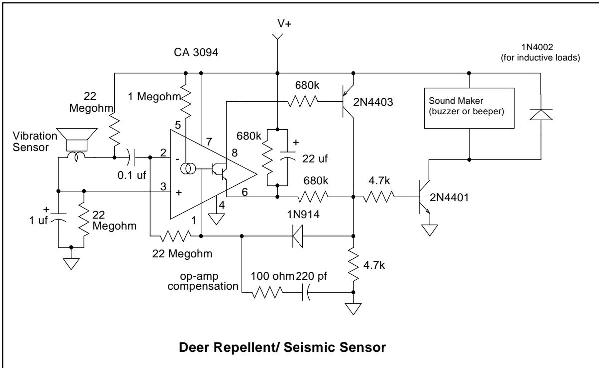
The unit is designed to consume minute amounts of power when not rattling to provide many months of unattended protection (practically set by the battery shelf life). The seismic sensor is built from an ordinary 2 inch speaker by gluing a mass to the speaker cone to lower its resonance frequency. A lid from a baby food jar with a little extra weight glued to the inside will work fine.
