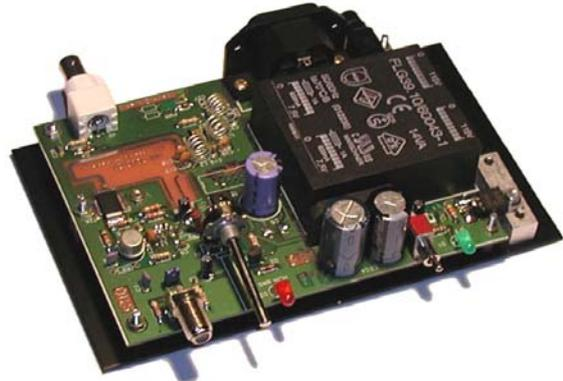
Fig. 1; 10W booster without the enclosure
