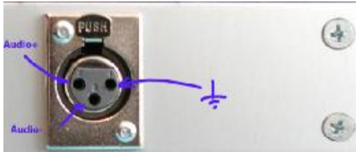
Figure 3: Balanced audio input – XLR input
