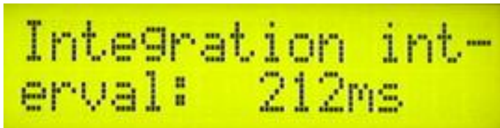
Figure 10: Setting the integration interval, this is the time the DSP extracts the samples
