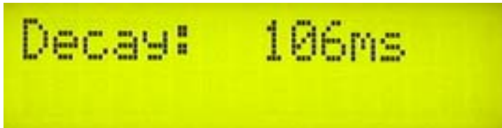
Figure 9: Setting the decay time, this is the time the compressor needs to respond to a decrease of the signal
